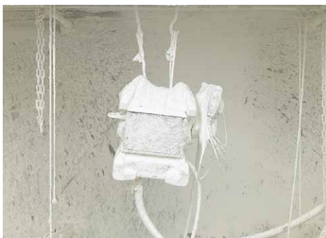
IPLEX FX under dust resistance testing
