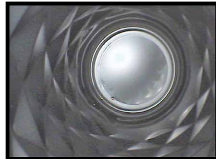
Image with WiDER™ gain applied. WiDER™ gain brightens the darker areas while maintaining the light level and details shown in the bright area.
